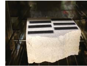
Figure 3: Thermal treatment of flexural test coupons
